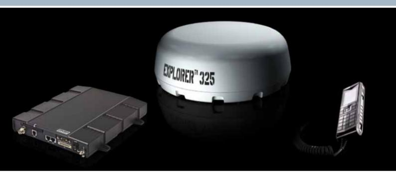
EXPLORER 325 has the smallest on-the-move BGAN antenna in the market. The system consists of three fully integrated units a transceiver, an IP handset and a roof mountable antenna.
